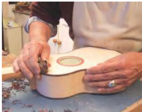
STEP 41. Trimming the bindings flush
